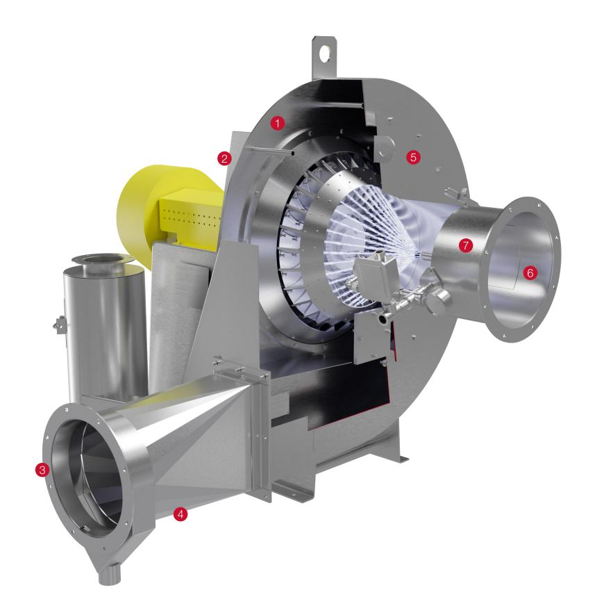
6 Rotating impellers cause particles to be impinged on and trapped by the flowing water film covering all surfaces of the blade.
